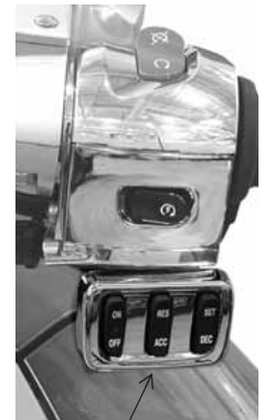
Cruise Control Switches
