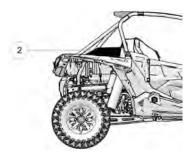
Inspect the engine pre-filter before each use of the vehicle to ensure adequate air flow. If necessary, remove the pre-filter and clean with soapy water. Dry with low pressure compressed air.
