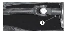
① Middle Prop Shaft Grease Fitting
